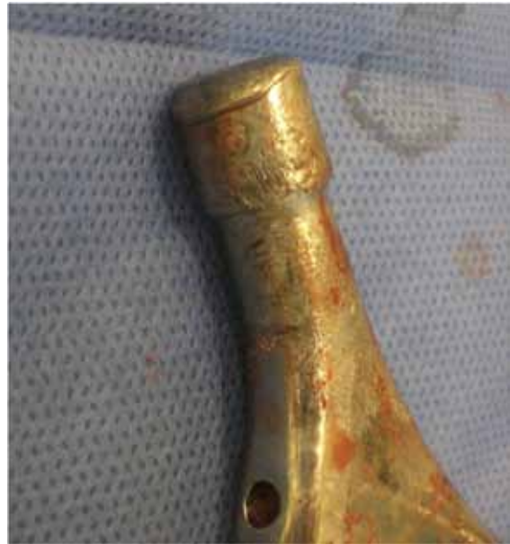
Figure 3. A. Remains of the fractured ceramic femoral head. B. Morse taper of the distorted femoral stem and the fractured femoral head.
