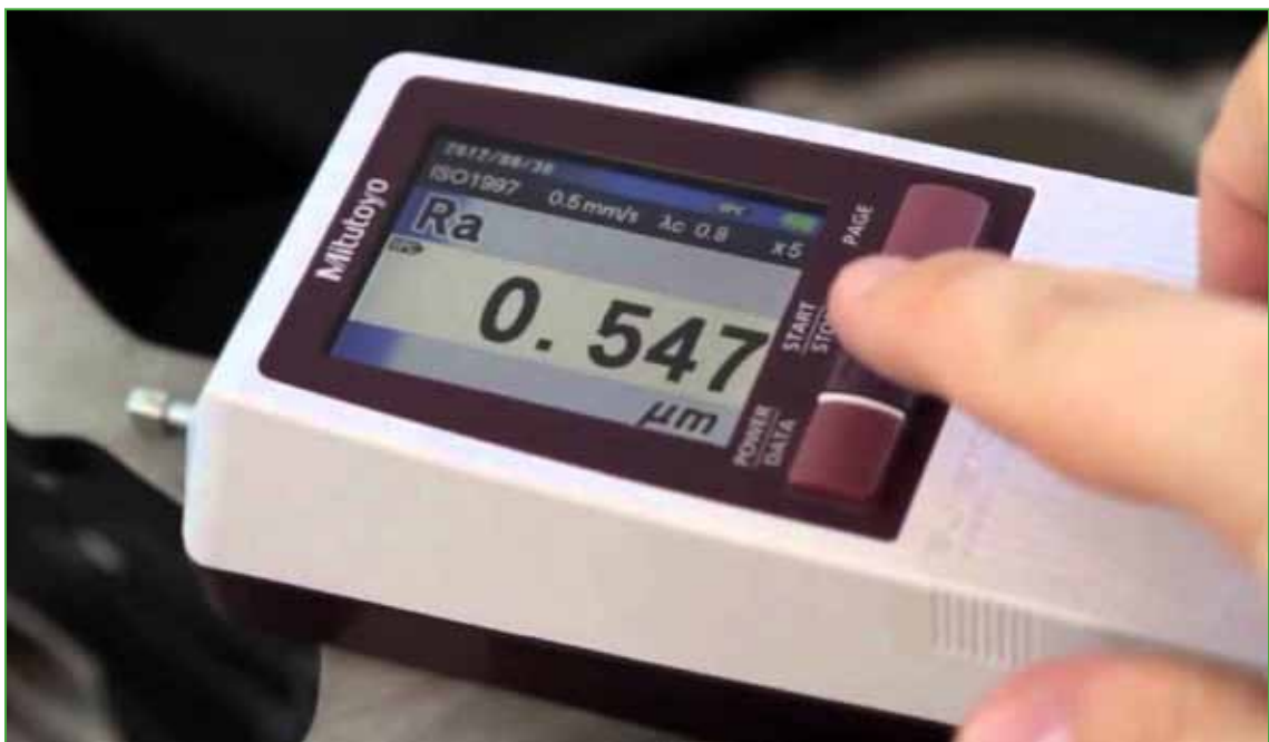
Figure 2. Mitutoyo surface roughness tester model SJ 210.
