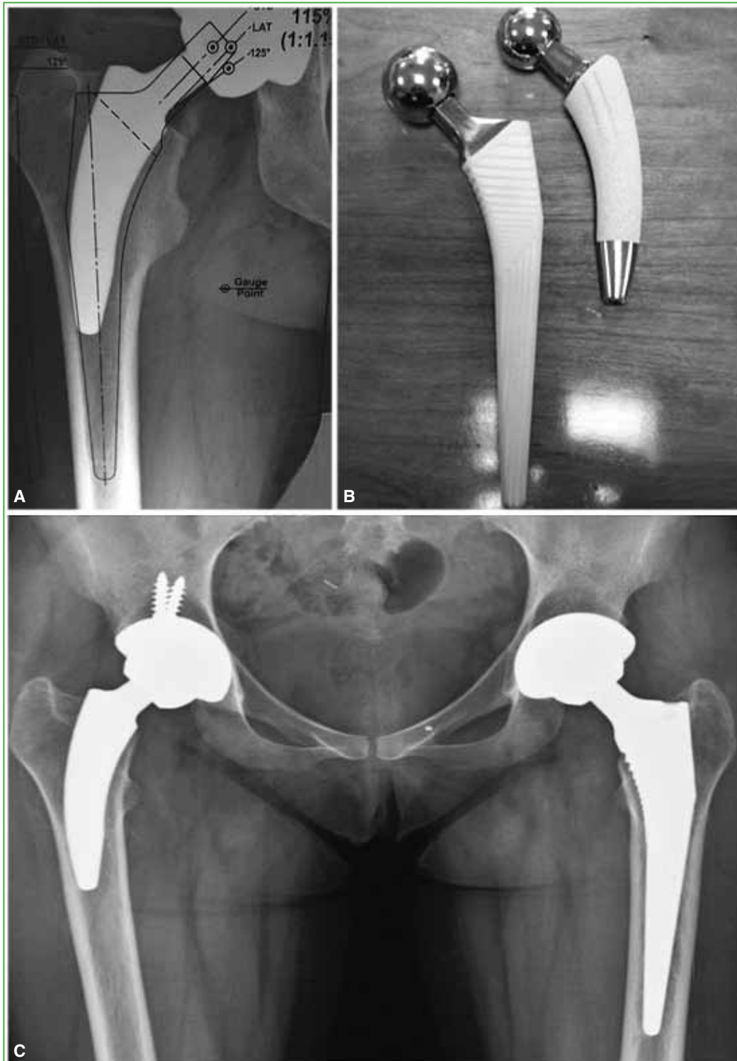
Figure 4. A. Measurement procedure with a postoperative anteroposterior radiograph of the hip. The neck cut level and the length of the implant that would have been placed in the case of using a metaphyseal-diaphyseal fixation stem are drawn. B. The two measured implants are shown: the cervicometafixation stem (on the right) and the metaphysodiaphyseal fixation stem (on the left). C. Patient with a cervicometafixation stem in the right hip and a metaphysodiaphyseal fixation stem in the left hip. Note the difference in length at the level of the neck cut and in the invasion of the femoral canal.
